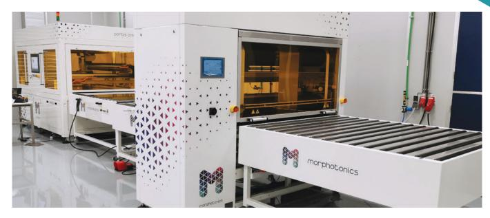
Portis 1100 is a modular Roll-to-Plate (R2P) nanoimprint equipment designed for R&D, process development, and production, with large-area capability. Portis 1100 offers a configurable and expendable nanoimprinting platform, combining Primer (P1100), Coater (C1100) and Imprint (NIL1100) modules.
