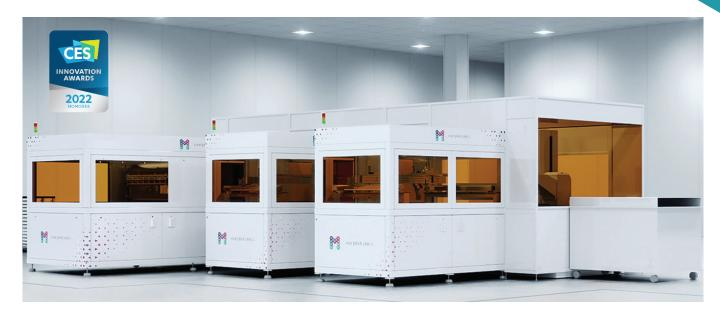
The Aurora Roll-to-Plate (R2P) nanoimprinting platform is a game changer for mass production. With its fully automated, highly accurate integrated modules working continuously, it can achieve imprint cycle times of under two minutes in mass production.
